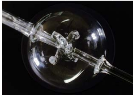
Perfectly Stirred Reactor
