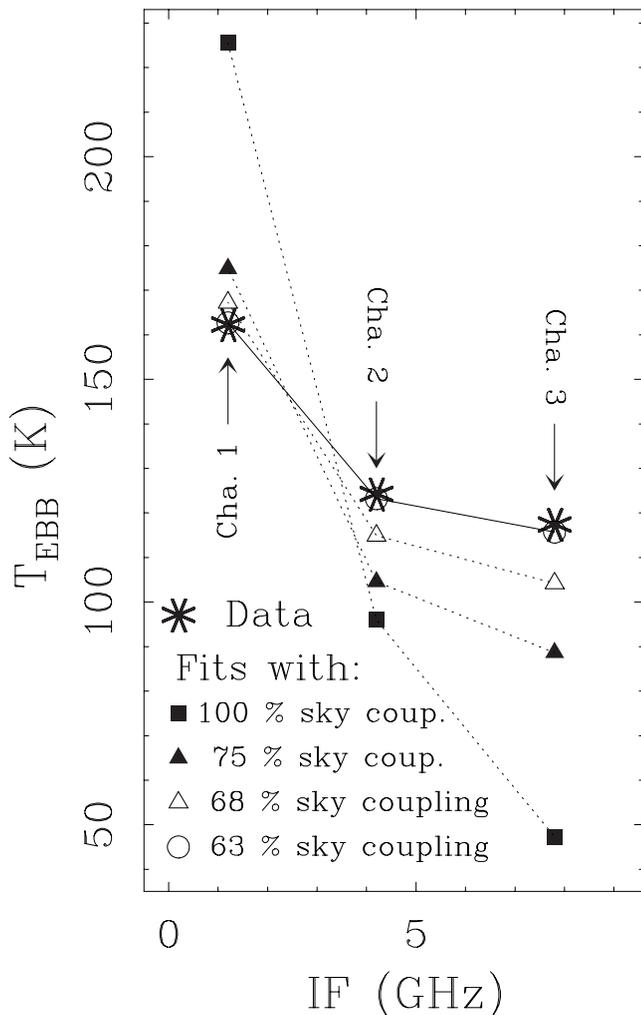
FIG. 2.—Fit of a set of WVM measurements from which the sky coupling of the instrument can be directly deduced. The signal is given in equivalent blackbody temperature ( $T_{\text{EBB}}$ ).
