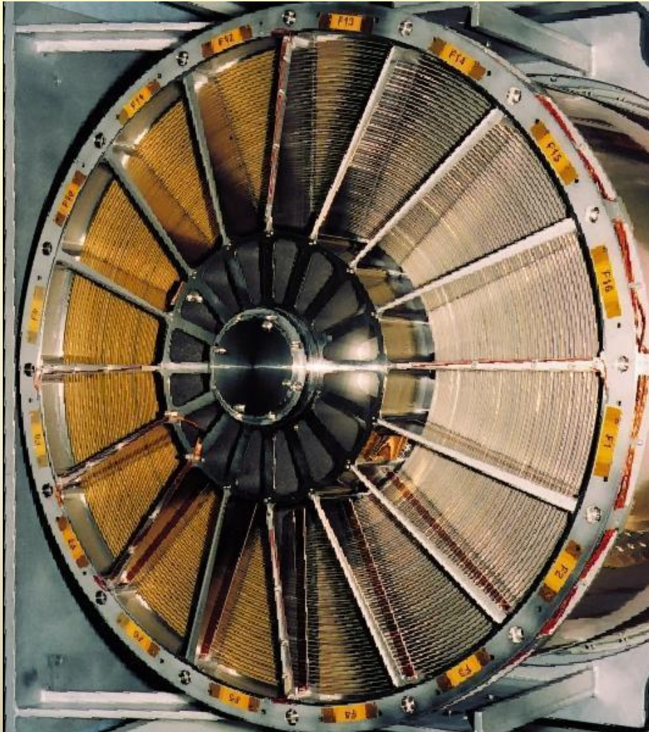
XMM-Newton mirrors during integration
