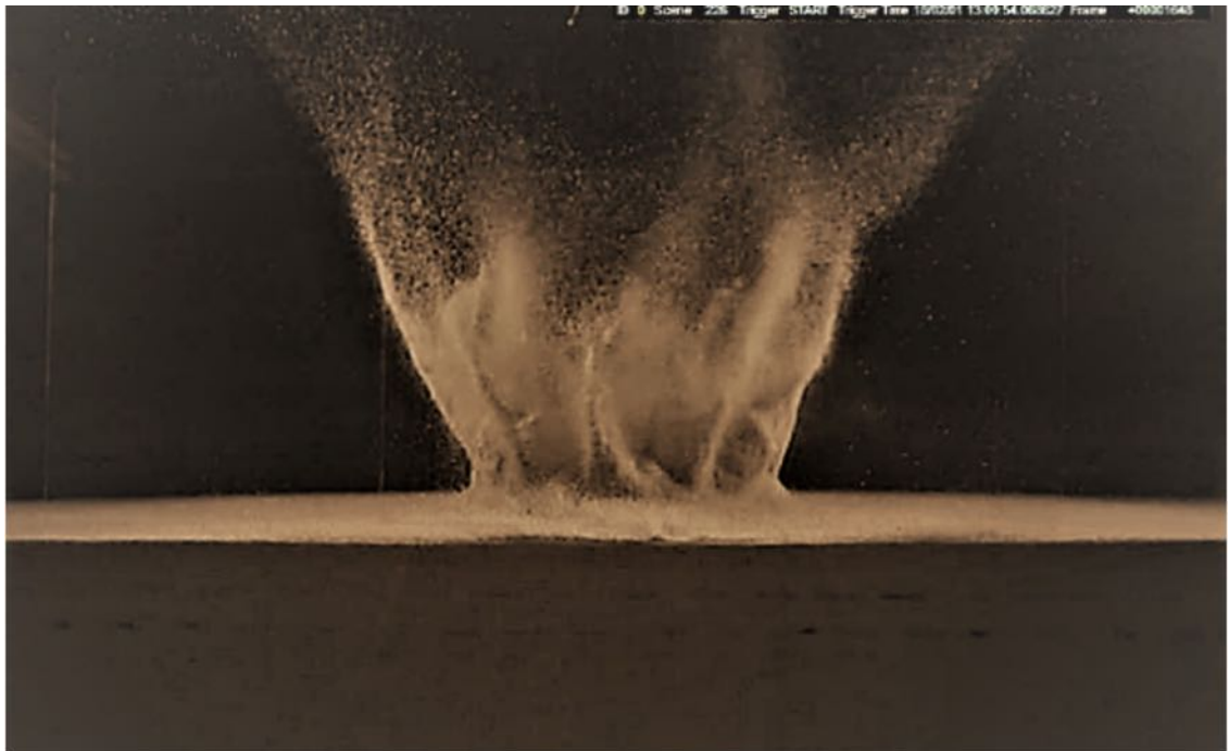
Figure 3: Half-space experiment in the Experimental Projectile Impact Chamber (EPIC) at the CAB INTA-CSIC showing an irregular ejecta curtain developing after the impact into a heterogeneous target consisting of sand with inter-bedded ceramic plates. Also the resulting crater and ejecta layer differ from an impact into a homogeneous medium. Width of frame 70cm.
